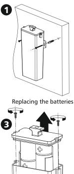
1 Drill two 6mm holes if drilling into a solid wall and insert the wall plugs. Screw the Battery Pack to the wall using the M4 x 40mm screws.
